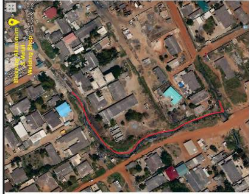
12 250.0m x 3.50m x 1.50m reinforced concrete drain at Nungua. (Redesigned to 250m x 3.0m x 1.8m rein. conc. drain-95% completed)
