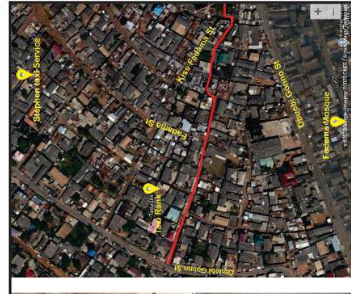
7. 250.0m x 3.50m x 1.50m reinforced concrete open drain at Abeka Lapaz (2018). (Redesigned to 350m x 2.0m x 1.3m rein.conc. drain -100% completed)
